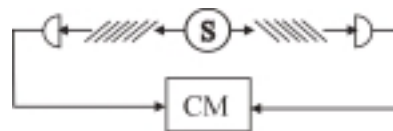
Fig. 2: Setup for “single-channel” Bell test
